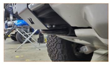
02. Insert the mounting plate into the bottom of the tow hook and, using (2) 10mm wrenches, secure it to the bolts with the supplied flat washers, lock washers, and nuts.
