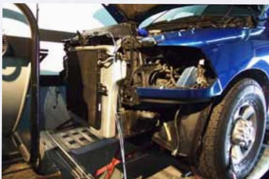
**Figure 8:** Dynamometer testing of the Mishimoto Intercooler
