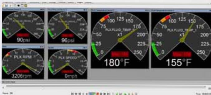
Air intake temperatures (AIT) were taken from the inlets and outlets of both intercoolers using PLX K-type thermocouples. Boost pressure was also tested to ensure that no dramatic pressure drop occurs when installing the larger Mishimoto intercooler.
