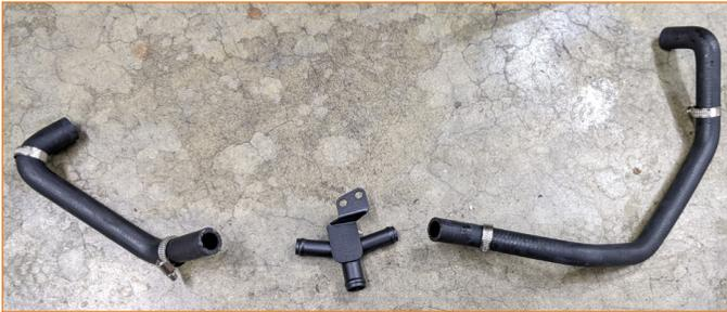
22. Install Y-pipe to passenger-side intercooler using supplied hardware.
