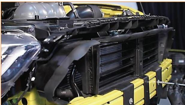
**36.** Reattach the ambient temperature sensor.
