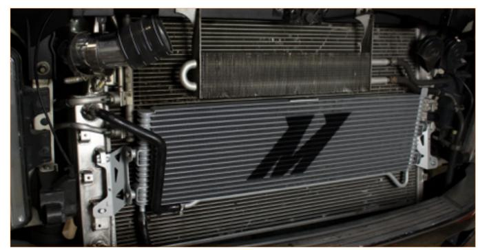
FIGURE 3: Mishimoto transmission cooler installed (intercooler off).
