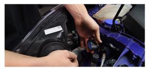
13. Pull up on the two tabs holding the front bumper. You can then lift the front bumper and slide it forward to separate it, but before completely removing the bumper, disconnect the fog light electrical connector.
