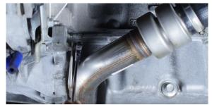
Loosen the clamp on the coupler between the hot-side pipe and turbo. (1x worm gear clamp)
