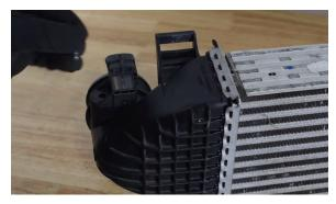
24. Install the sensor removed from the stock end tank onto the Mishimoto intercooler. Secure it with the bolt from your kit.(1x T25 torx bolt)
