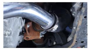
Align the pipe so it will fit in the crease between the transmission and oil pan without touching either. Rest the two brackets welded to the pipe on the studs you removed nuts from earlier. Secure the pipe with those original nuts. (1x 10mm nut, 1x 13mm nut)
