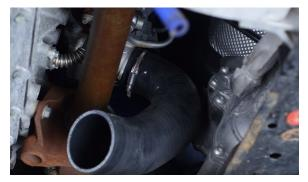
Install the intercooler pipe to the open end of the coupler you just installed to the turbo. (1x worm gear clamp)
