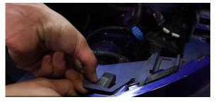
14. Remove the upper air shroud by releasing the two clips that hold it in place.
