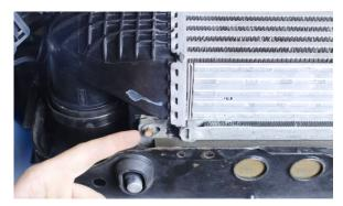
21. Use a pick tool to loosen the connection between the pipes and end tanks on the intercooler. Then, slide each pipe off the port.
