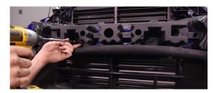
Disconnect the electrical connector for the active grille shutters, and then pull out the tree-clips holding the wire. (2x tree clips)
