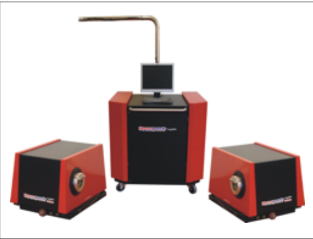
FIGURE 3: A Dynapack dynamometer was used to apply a repeatable load on the Focus ST during testing.
