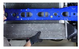
23. Remove the sensor from the end tank on the stock intercooler. (1x T25 torx screw)
