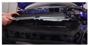
15. Remove the lower air shroud, which is held by two screws.
