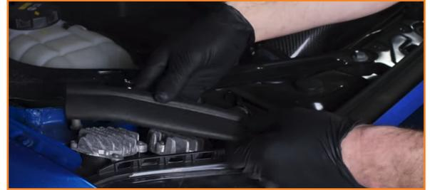
3. Remove the bolts on the upper portion of the bumper. (6x T27 torx bolts)
