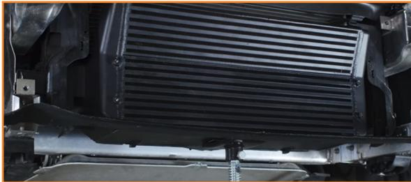
20. Attach the cold and hot-side pipes to the intercooler end tanks. (2x spring clips)
