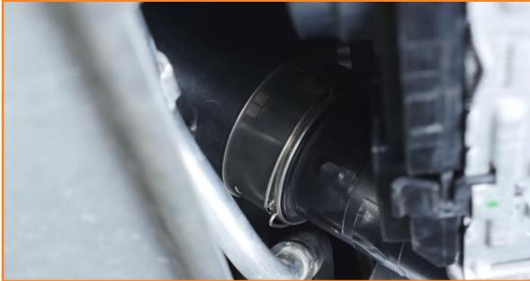
17. Remove the bolts on the bottom of the intercooler. Support the intercooler with your off hand to prevent it from falling. (2x T25 torx bolts)
