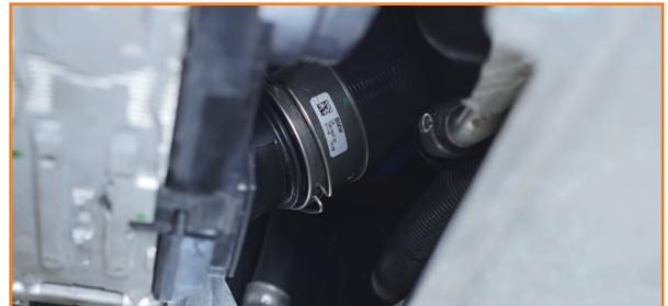
16. Disconnect the cold-side pipe from the intercooler end tank. (1x spring clamp)
