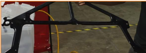
22. Reinstall the bracket over the intercooler. (6x T45 torx bolts)
