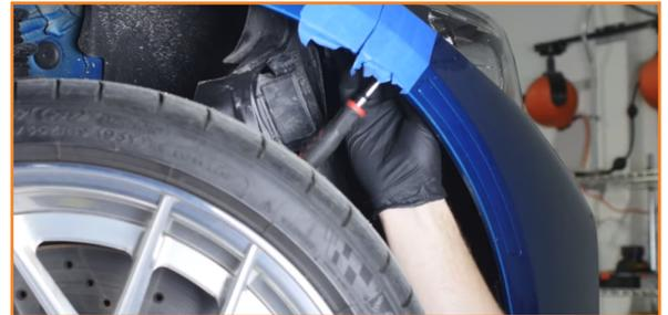
7. Pull back the fender liner to expose the driver-side wheel well.
