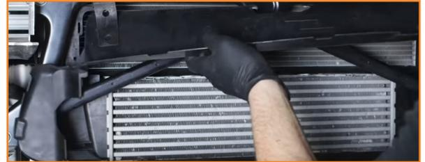
14. Remove the bolts that secure the bracket covering the intercooler. Two of the bolts can be found within the top edge of the engine bay. (6x T45 torx bolts)
