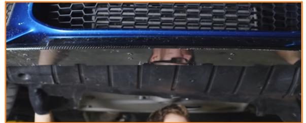
5. Pull back the fender liner to expose the passenger-side wheel well. (3x 8mm screws)
