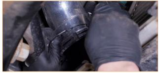
07. Loosen the clamps that secure the Y-shaped induction hose to the airbox and intake pipes. Then separate the induction hose from each connection and remove it from the vehicle. (3x worm-gear clamps)
