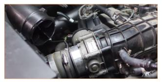
**05.** Disconnect the wiring harness from the sensor on the cold-side intercooler pipe. To release this connector, depress the black tab and pull the connector off the sensor.
