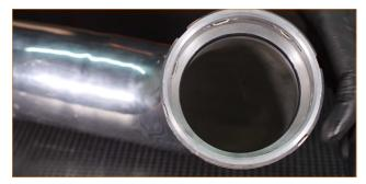
**37.** Lift the bottom section of the cold-side pipe into place and install it to intercooler outlet. Make sure the circlip engages the slots on the hot-side pipe. The clip should snap into place when you press the pipe down over the intercooler outlet. (1x circlip)
