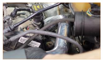
19. Locate the single-bend, long coupler included with your kit. Identify the smaller end of the coupler and install a 63–70mm clamp over this end. Then lower the coupler into place and slip it over the pipe you just installed. (1x T-bolt clamp)
