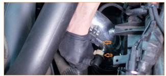
10. Loosen the clamp that secures the cold-side intercooler pipe to the throttle body. Then separate the pipe from the throttle body. Lift the pipe upwards to give yourself more room around the intercooler. (1x worm-gear clamp)
