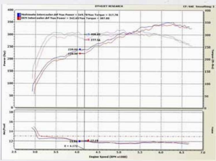
Figure 5: Dyno graph comparing OEM intercooler and Mishimoto intercooler power curves. The Mishimoto unit easily supported 350 whp and is capable of yielding much more power with a proper tune and supporting modifications.
