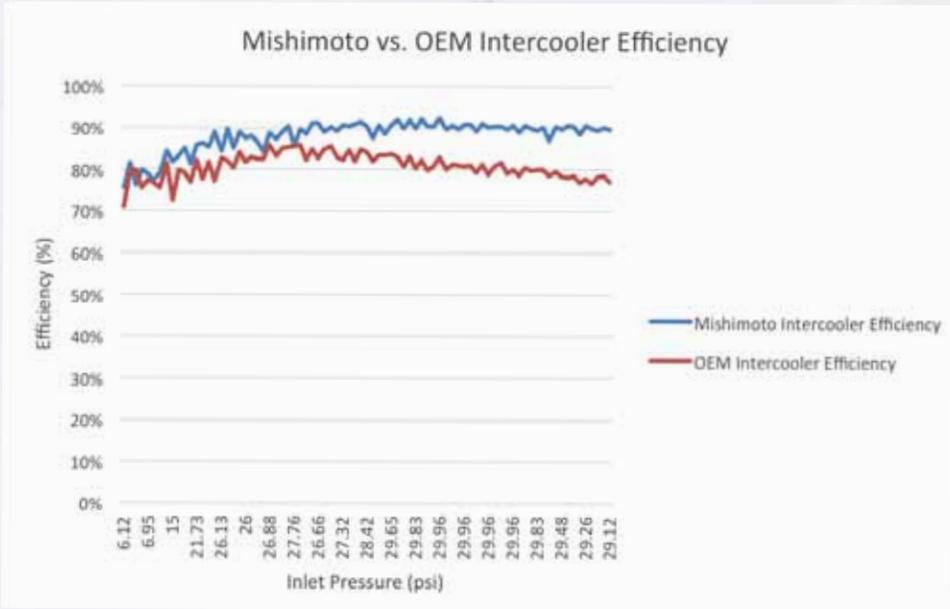
**Figure 3:** As inlet pressure increases, the efficiency of the Mishimoto intercooler increases dramatically compared to the OEM unit. A higher efficiency means the unit has greater heat transfer properties and will allow colder air to enter the motor. In general, colder air allows the engine to make more power.
