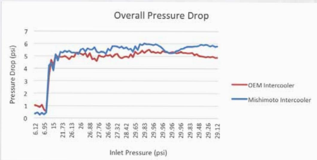
**Figure 4:** The Mishimoto intercooler shows little increase in pressure drop compared to the stock unit.
