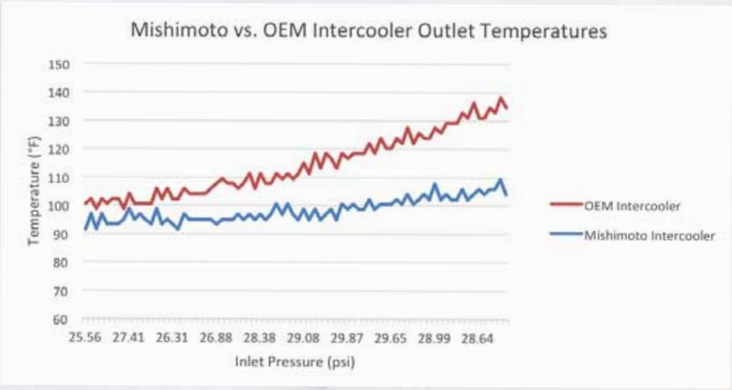
**Figure 2:** The OEM intercooler showed an average temperature of 113.6 degrees. The Mishimoto unit showed an average temperature of 99.4 degrees. This colder intake air allows for a more aggressive tune which will result greater power.
