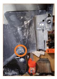
Remove the plastic cover in the passenger-side wheel well.(1x pop clip)
