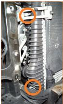
**29.** Remove the bolts securing the radiator to the intercooler. [4x 13mm bolts]
