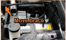
17. Remove the bolt securing the brace to the upper core support and loosen the bolt securing the brace to the driver-side fender. Move the brace away from the upper core support. (2x 10mm bolts)
