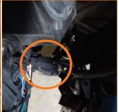
**11.** Remove the headlights. (4x 10mm bolts and 1x electrical connector on each side)
