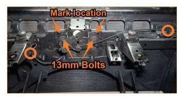
14. Using a marker or scribe, mark the location of the hood latch. Remove the hood latch from the grille support and place it to the side. [2x 13mm bolts, 1x harness tree clip, 1x hood latch cable routing tree clip]
