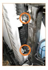
**30.** Remove the grommets from the driver-side brackets on the radiator. (2x grommets)
