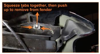
**12.** Remove the threaded headlight mounting clips from the fenders. (1x mounting clip on each side)
