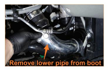
**27.** Remove the cold-side intercooler pipe lower section from the vehicle. (1x constant tension T-bolt clamp)
