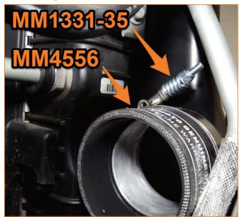
**42.** Connect the larger diameter of the MM4556 boot to the cold-side of the intercooler as shown in the image above. (1x MM4556, 1x MM1331-35 constant tension t-bolt clamp)
