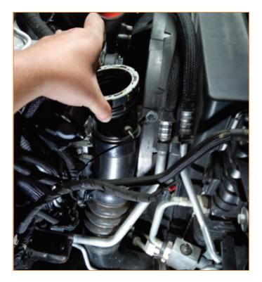
24. Remove the stock cold-side pipe from the vehicle.
