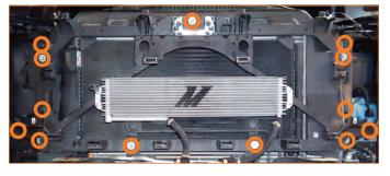
15. Remove the grille support from the vehicle. (7x 13mm bolts, 6x 10mm nuts) \*\* If you have the Mishimoto transmission cooler kit installed on your vehicle, you'll need to disconnect the hoses from the cooler.\*\*
