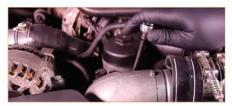
03. Apply high-tack gasket sealant to the groove in the Mishimoto intake elbow where the O-ring will be seated, and allow it to set up for a moment.
