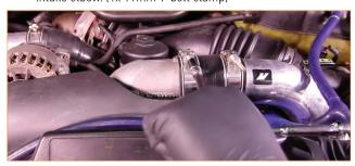
02. Unbolt and remove the stock intake elbow. [4x 8mm bolts.] 1x 12mm nut)
