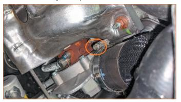
**06.** Unplug and remove the blow-off valve from hot-side pipe. (3x 8mm plastic screws, 1x tree clip)
