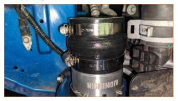
**12.** Install the aluminum pipe section and secure it to the engine block with the original 13mm bolt you previously removed. Do not fully tighten.
