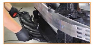
Remove the bolts that secure the hot and cold-side pipes to the intercooler end tanks. (4x 10mm bolts)
