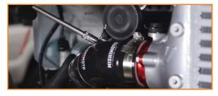
37. Install the plastic ducting that comes in your kit to the intercooler as shown here.
