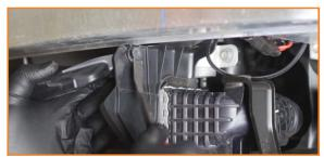
2. Release the top panel portion of the intercooler ducting. (2x pop-clips)
