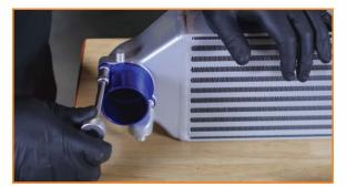
Lift the intercooler into place. Engage the pegs on the end tanks with the grommets. Connect the cold-side hose to the end tank and secure the connection with the provided clamp. (1x worm gear clamp)
