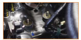
23. Install the cold-side pipe. You will want to first connect it to the silicone hose on the throttle body. (1x worm gear clamp)
