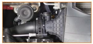
4. Separate the brackets holding down the intercooler end tanks. (2x 10mm bolts)
