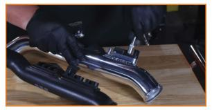
20. Transfer the hardware and bushings from the stock pip over to the Mishimoto hot-side pipe.
