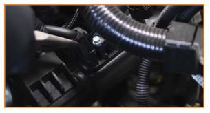
16. Loosen the clamp on the cold-side pipe and throttle body connection. (1x worm gear clamp)
