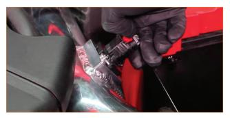
**07.** Remove the airbox isolator bushing. Remove the screw that runs through the center of the bushing. Then remove the bushing by pulling it upward. (1x T20 Torx screw)
