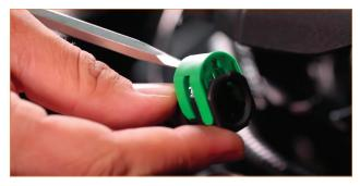
05. Loosen the two clamps that secure the rubber intake hose to the airbox and the intake tubing. Remove the rubber intake hose from the vehicle. (2x worm-gear clamps)
