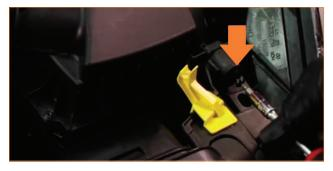
08. Separate the air intake duct from the radiator support by prying up on the edge near the center of the duct. Remove the air intake duct and airbox as one unit by pulling the airbox upward. The airbox is secured to the vehicle with two rubber grommets.
