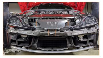
07. Remove front bumper bolt bracket. (4x 10mm bolts)
