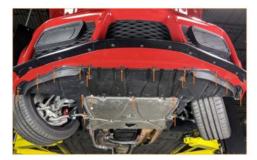
**04.** Disconnect the two electrical connections on the driver and passenger side just below the headlight near the wheel.
