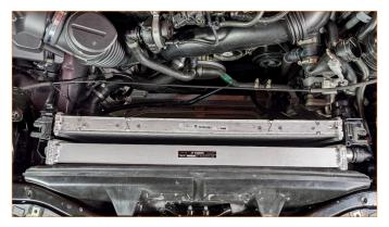
27. Reconnect the quick disconnects supply and returns on both the radiator and the heat exchanger. Ensure the locking ring is securely in place. Reattach the sensor's electrical connection on the back right side of the radiator.
