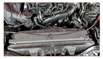
12. Remove the lower radiator cover in the same manner as the upper cover. Be careful where the inlet to the heat exchanger is you may need to use a pick tool to release a plastic tab up above the inlet. See dashed arrow. (2x T30 plastic screws)
