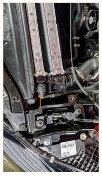
17. Remove the sensor wire from the back of the radiator.
