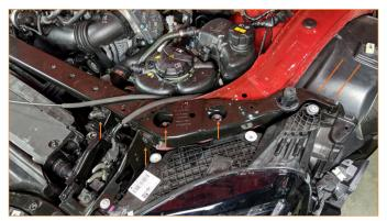
To remove the fan shroud, disconnect the electric plug on the back of the fan and remove plastic screws that secure it to the top of the radiator. (2x T30 screws)
