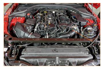
Reattach the transmission cooler. Slide tabs on the Mishimoto heat exchanger, then secure in place using 2.5mm allen tool. (2x M4X0.7 bolts)
