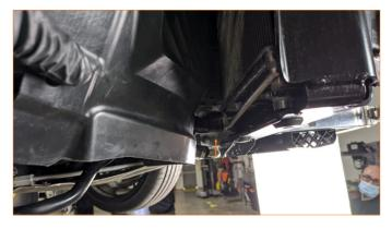
**14.** Drain the secondary cooling system by removing the lower quick disconnect from the heat exchanger.
