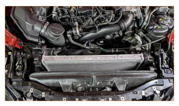
26. Next, slide the heat exchanger down from the top. This can be done without removing the radiator once all plastic pieces have been trimmed.
