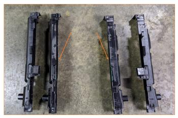
This cutting can be performed on the vehicle without removing the radiator. However, for demonstration and easier cutting, removing the rad and pieces from the vehicle was done.
