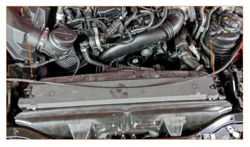
**31.** Reinstall the upper crossbar. Take special note of where the hood release lines go. (4x E14 bolts, 4x 13mm bolts, 4x 10mm bolts)
