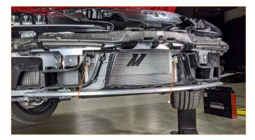
Reinstall the stone guard using the provided hardware and brackets. (2x brackets, 2x M4X0.7 bolts)
