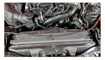
Remove the upper radiator cover. Simply unclip and pull off. (2x T30 plastic screws)
