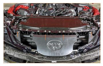
Remove the top metal radiator cover. Lift out of place once bolts are removed. (13x 13mm bolts)
