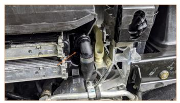
**15.** Remove the radiator hoses by releasing the clips that hold the quick disconnects to the radiator.
