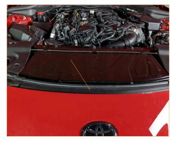
02. Remove fender tops from driver and passenger side of vehicle. Hardware is shown on passenger side below. Locations are mirrored in location on the driver's side. (8x Pop-clips)
