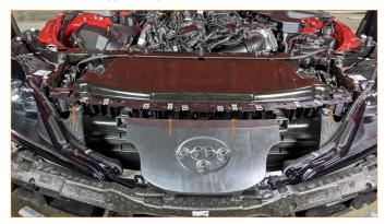
Reinstall the front bumper support. This is held in place with 2X T30 bolts (top) and 2X T30 plastic screws (bottom).
