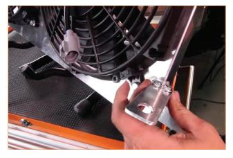
25. There are two holes along the upper edge of the fan shroud. Install the long dowel to the hole closest to the corner of the fan shroud, but do not fully tighten. Install the short dowel to the hole farthest from the corner on the fan shroud, but do not fully tighten. (2x 10mm bolts, 2x dowels)
