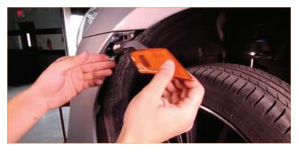
Remove the pop-clip behind the side marker light; it connects the bumper cover to the fender. Do this on both sides. (2x pop-clips)
