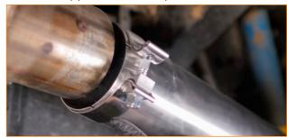
05. Locate the long section of exhaust, hardware, and bolt-on hanger in your kit. Slip the washers over the bolts and install the hanger to the exhaust system as shown here. Leave the bolts loose for now; we will tighten them later when adjusting the exhaust fitment. (2x 17mm bolts, 2x lock washers, 2x flat washersl
