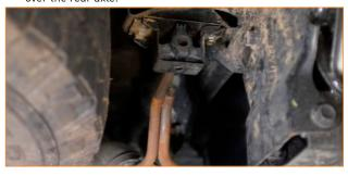
04. Locate the short, straight section of exhaust in your kit. Slip one of the provided worm-gear clamps over the front of this section and install it to the DPF. Then tighten the clamp to secure the pipe. (1x exhaust clamp)
