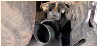
08. Slip an exhaust clamp over the long section. Locate the last exhaust pipe in your kit and install it to the long section. Slide the pipe on until it is fully seated, but leave the clamp loose for now. (1x exhaust clamp)
