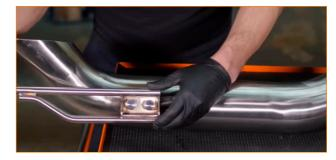
06. Slip a clamp over the straight section you just installed. (1x exhaust clamp)
