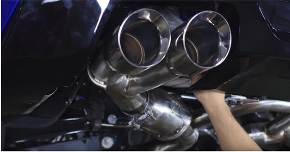
13. Check that all pipe connections are fully seated. Then properly position the clamps over each connection and tighten them down.
