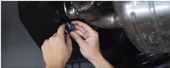
5. Remove the nuts that secure each rear exhaust mount. (4x 15mm nuts)
