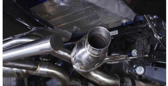
10. Align the brackets on the resonators to secure them with the bolts from your kit. Leave the bolts loose for now.
