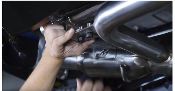
11. Transfer the rear exhaust mounts from the stock exhaust hangers to the Mishimoto tips.
