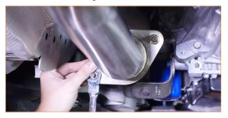
O8. Slide a clamp over the front pipe you just installed. Then install the mid pipe over the open end on the front pipe. (1x exhaust band clamp)
