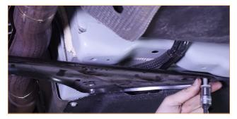
02. Remove the two nuts from the flange that attaches to the downpipe. (2x 15mm nuts)
