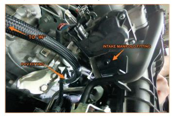
9. Install on end of the SHORTER hose onto the intake manifold fitting and the other end to the "OUT" fitting on the catch can. If you prefer to use the optional clamps, make sure to install 2x clamps on the hose BEFORE installing the hose. NOTE: Pay special attention when removing this hose in the future as the intake manifold fitting can easily break off from the intake manifold.
