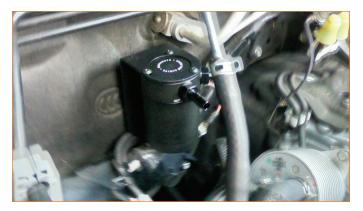
**12.** Reinstall intake tube. DO NOT forget to reattach the hose on the back of the tube.
