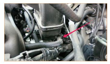
**3.** Remove Factory PCV line that connects the back of the intake manifold (behind throttle body) to the PCV fitting on the block.
