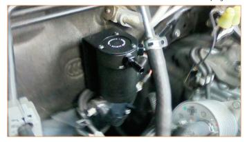
8. Take the LONGER of the two hoses and attach one end to the PCV fitting on the block and the other end to the "IN" fitting on the catch can. If you prefer to use the optional clamps, make sure to install 2x clamps on the hose BEFORE installing the hose.
