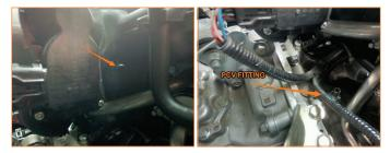
4. Locate and remove two 10mm bolts on the firewall. The lower one secures a plastic wire cover and the upper bolt secures a ground wire. Take special care to make sure that the bolts go back into the same holes (the lower bolt has the cross for phillips-head screwdriver).
