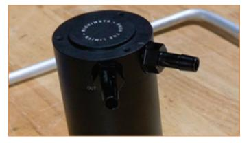
**7.** Install the catch can onto the bracket as shown. The outlet ("out") of the catch can should be facing approximately towards the front of the vehicle. Thread the 3x 2.5mm allen head bolts but D0 N0T fully tighten.
