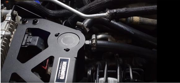
18. Install the hose from the intake manifold to the catch can's OUT port and secure it with the last of your smaller clamps. (1x worm gear clamp)
