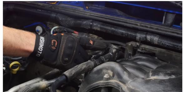
5. Loosen the two bolts on the ECU to make room for the catch can bracket. (2x 8mm bolts)
