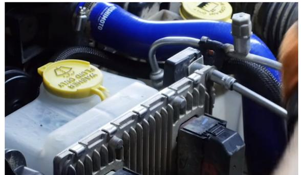
6. Loosen the bolt on the ABS control unit to make room for the catch can bracket. (1x 10mm bolt)
