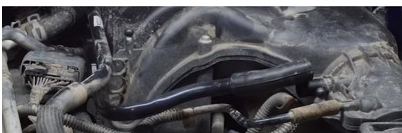
3. Separate the PCV hose from the intake manifold.
