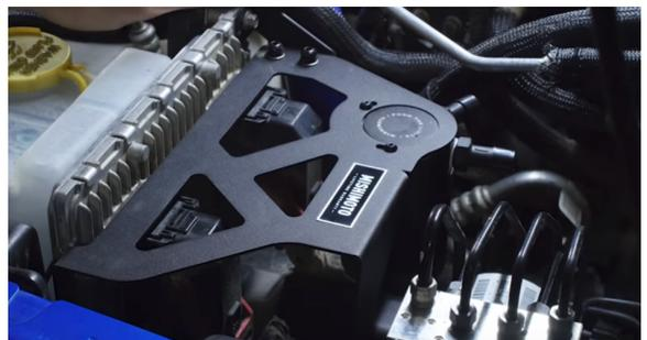
17. Install the hose from the PCV valve to the catch can's IN port and secure it with one of the smaller clamps. (1x worm gear clamp)
