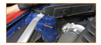
3. Loosen the nut on the passenger side strut tower,
