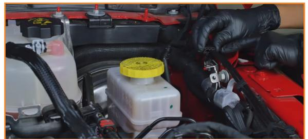
4. Loosen the two bolts on the fender, leaving enough room to fit your bracket. (2x 16mm bolts)
