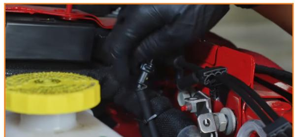
6. Install the bracket over the two bolts you loosened. (2x 16mm bolts)
