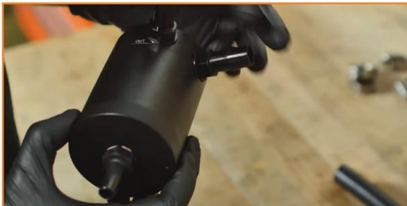
10. Attach the drain kit hose to bottom port. Use a smaller clamp here. (1x worm gear clamp)
