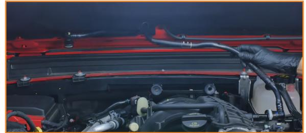
3. Free the washer fluid line's clip that's secured to the bracket. (1x tree clip)
