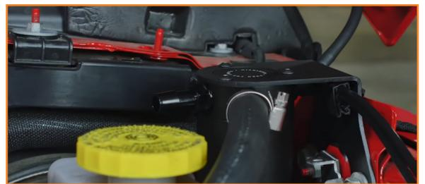
18. Connect the quick-disconnect on the shorter hose to the intake manifold.
