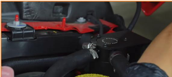
20. Reinstall the engine cover. Slide the back end in first and lower the front end in place. (2x 10mm bolts)
