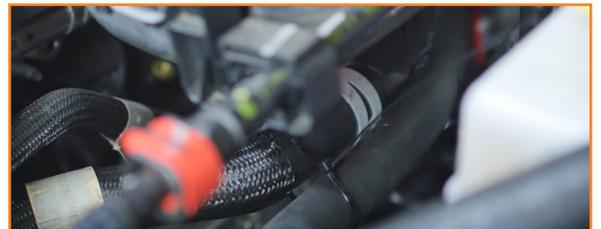
17. Install the open end of the hose to the catch can's IN port. (1x worm gear clamp)
