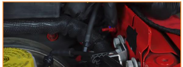
5. Use a zip tie to secure the loose washer fluid line.
