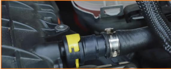
19. Install the open end of the shorter hose to the catch can's OUT port. (1x worm gear clamp)
