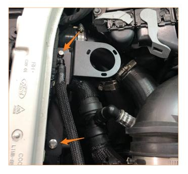
04. Remove the 3X M4 allen-head screws from the catch can using a 2.5mm allen key. Install the two catch can fittings in the catch can using a 17mm wrench. Install the catch can on the bracket as shown, leaving the 3X allen head screws loose.
