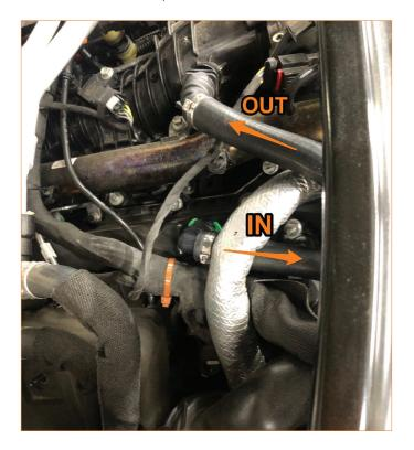
07. Adjust the rotation of the catch can and tighten the 3X M4 allen bolts with a 2.5mm allen key.
