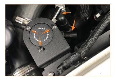
**05.** Take the longer hose with the 45-degree fitting on it and connect the fitting side to the intake manifold, then route the hose underneath the intake tube. Connect to the "OUT" fitting on the catch can and secure with hose clamp. Verify that the hose is not rubbing on the intake tube. You may need to loosen the hose clamp and rotate the hose on the fitting to make sure that it has clearance away from the intake hose.
