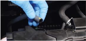
Remove the two bolts securing the cover over the fuel line. (2x 10mm bolts)
