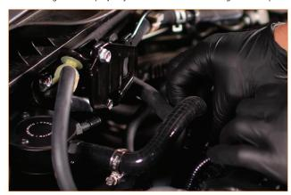
14. Locate the straight Mishimoto hose. Install one of the provided worm-gear clamps over each end of this hose. Install one end of this hose to the port marked IN on the catch can. Then install the other end to the port on the valve cover. Secure the hose with the worm-gear clamps you just installed. (2x worm-gear clamps)
