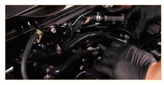
**15.** Now go back and fully tighten the Allen bolts that secure the catch can to the mounting bracket.
