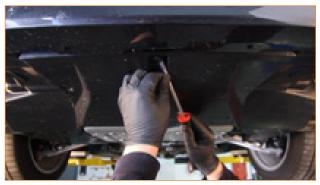
**6.** Remove the clips holding the undertray to the aluminum plate (4x small pop clips)
