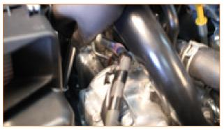
**16.** Remove the hold-down bracket nuts for the intake (2x 10mm nuts)
