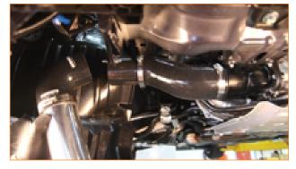
2. Tighten the engine side clamp (1x worm-gear clamp)
