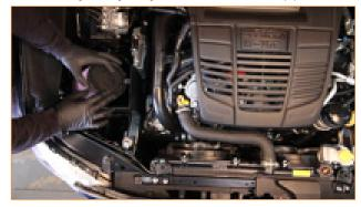
6. Tighten down the clamp (1x worm-gear clamp)
