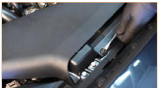
${\bf 2.}$  Loosen the intake hold-down bracket on the passenger side fender at the top of the airbox (2x 10mm nuts)
