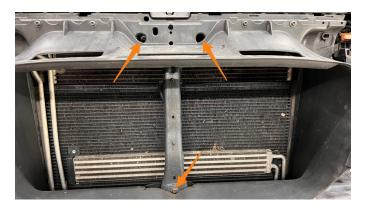
21. Remove the 8x Torx screws (T30) then pull the radiator air duct out.
