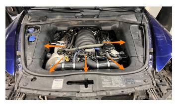
23. Disconnect the MAF sensor plug (1), pull the 2x pins for airbox intake pipe (2) and remove airbox lid (3) by releasing the 2x latches on the top. Remove the air filter and set aside in a clean spot. Repeat for the other side.
