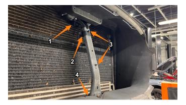
20. Remove the 3x Torx screws fastening the bracket (T30).
