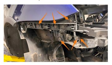
**43.** Remove the electrical connector from the headlight bracket by depressing the tabs and pulling straight up. Repeat for the other side.
