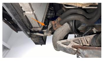
**37.** Reinstall the lower brace hand tight to support the cooling stack for the next steps.
