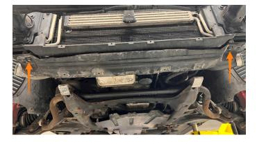
**38.** Use a pick tool to remove the metal clips from the rad mounts and then remove the black plastic caps.
