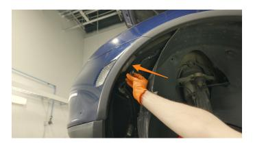
**9.** Remove the 2x Torx screws fastening the bumper (T30). Repeat for the other side.
