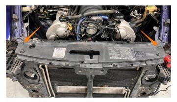
46. Remove upper rubber seal and mounts.
