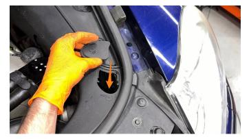
11. Rotate the hex drive clockwise (6mm socket). This will release the headlight and push it out slightly. The headlight can now be removed straight out the front. Repeat for the other side (rotation will be opposite).
