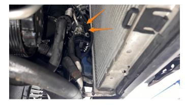
**35.** Remove the Torx screw (T30) fastening the power steering cooler lines to the radiator.
