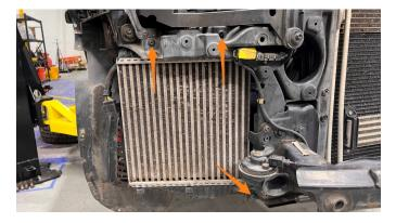
**28.** Disconnect electrical plugs for MAP sensor and throttle body, pull the 2x pins and remove Y pipe.
