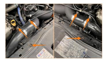
27. Remove the 3x Torx screws for the intercooler (T30) and pull the intercooler/pipe assembly out the side of the vehicle. Repeat for the other side.
