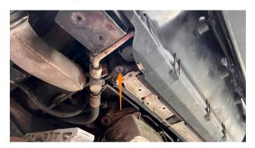
**16.** Disconnect the lower intercooler quick connect fitting by releasing the clip with a pick tool then pulling the charge pipe out. Repeat for the other side.
