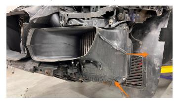
14. Remove the 4x bolts (13mm) then remove the brace to gain access to the radiator drain.
