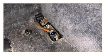
3. Under the vehicle, remove the 5x Torx screws (T25) then, remove the passenger side air duct. Repeat for the other side.
