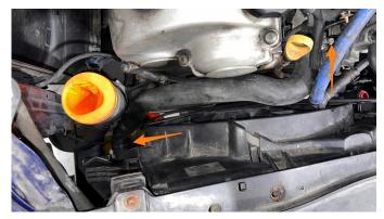
32. Loosen hose clamp (8mm) and remove upper hose.
