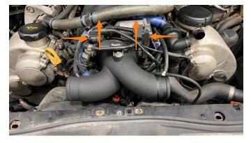
29. Release the fan shroud locks by using a screwdriver to push against the lever then lift the fan shroud up slightly out of the slots.
