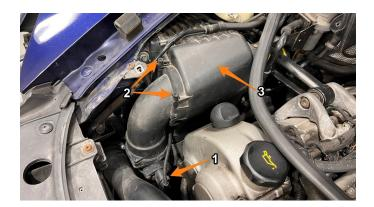
**24.** Loosen the hose clamp (8mm) and remove the top of the intake pipe. Repeat for the other side.
