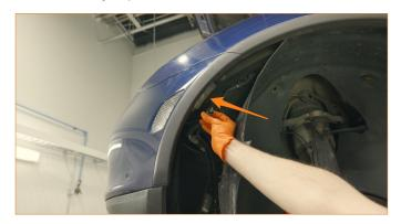
**8.** Unplug the electrical connector for the bumper harness on the passenger side.
