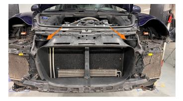
19. Disconnect the electrical connector from the hood latch (1), remove air temp sensor from bracket (2), and pull harness off bracket (3). Tuck the harness through the hole in air duct (4).
