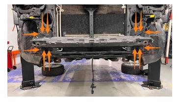
41. Remove the 2x upper rad mount Torx screws (T30).
