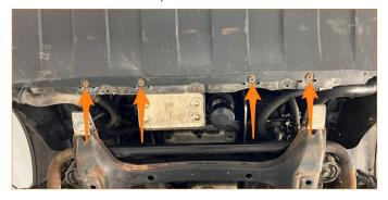
**6.** Remove the 6x Torx screws from the wheel liner (T25). Wheel removed for illustration purposes.
