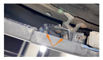
**10.** Remove the plastic cover by pushing down on the front-facing side.
