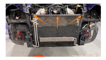
47. Zip-tie the top of the radiator to the frame to hold it in place then remove the lower brace that was reinstalled in step 37. Remove the clips holding the transmission cooler and AC condenser from the radiator.
