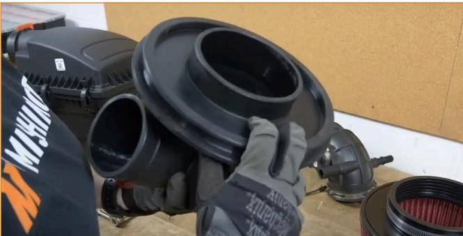
26. Slide the air filter over the intake tube. (1x worm gear clamp)
