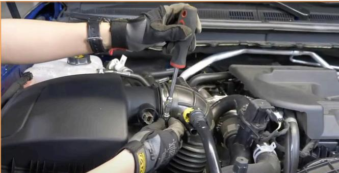
08. Remove the intake tube.
