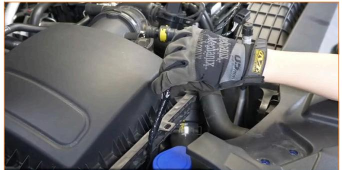
05. Separate the quick-disconnect by pulling the yellow tab out.
