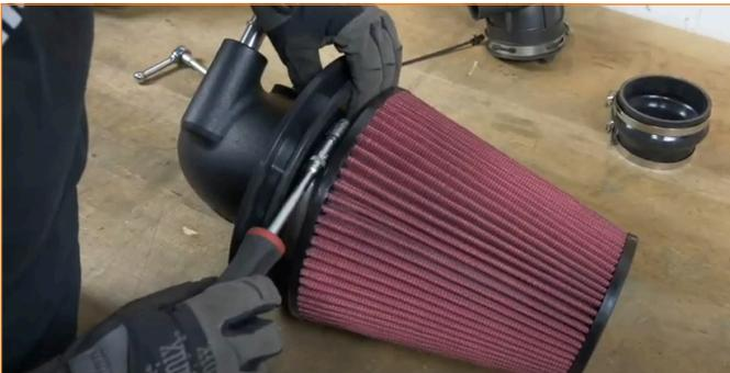
27. Place the smaller end of the intake coupler over the intake.
