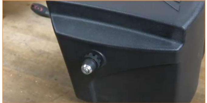
21. Install the airbox by aligning the side peg first, then the bolt holes.
