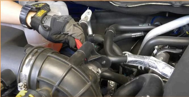
07. Loosen the clamps on either end of the intake tube.
