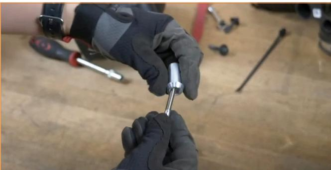
19. Install the assembled peg into the Mishimoto airbox. (5mm Allen key)
