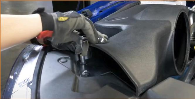
25. Slide the intake grommet over the intake tube with the words facing out.
