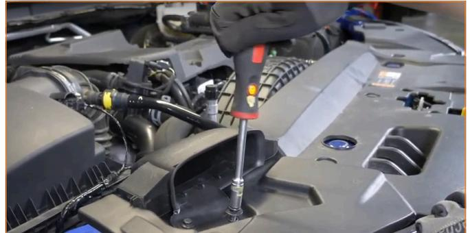
03. Disconnect the air intake sensor and condenser sensor.
