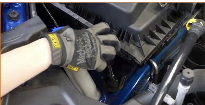
10. Lift the airbox and push toward the engine to disengage the rubber grommet.
