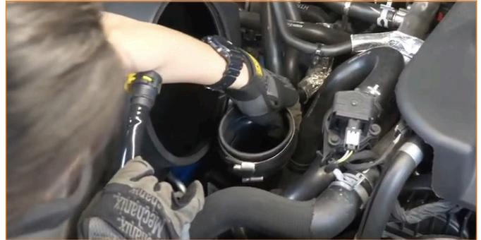
28. Slide the intake filter in first, and then rotate it to align with the coupler.
