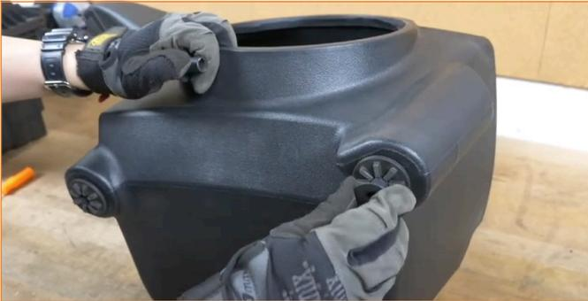
17. Remove the side grommet from the stock airbox.
