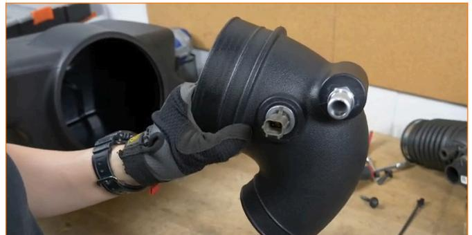
14. Remove the two inserts and grommets from the stock airbox.
