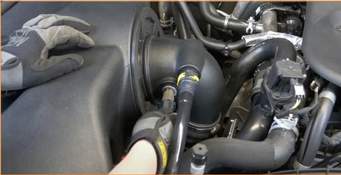
33. Wrap and secure the provided zip tie around the blow-off valve hose. Now attach this zip tie to the tree-clip zip tie that is already mounted on the coolant hose. The tree clip on the stock zip tie will push into the hole on the provided zip tie.
