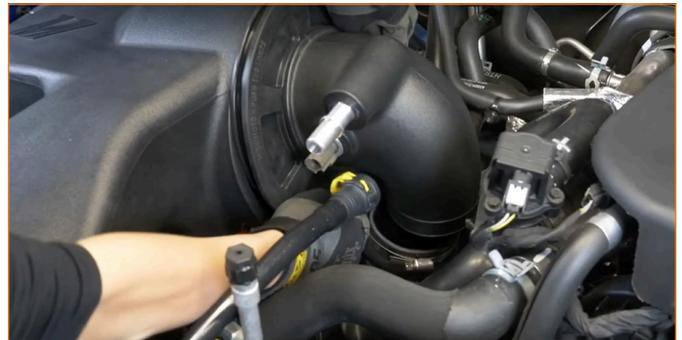
29. Once aligned, push the rubber grommet into place.
