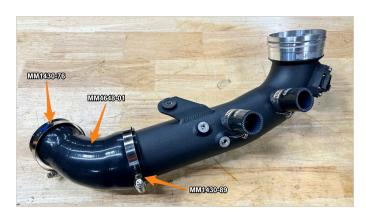
5. Install the charge pipe assembly into the vehicle throttle body side first. Push the pipe into the quick-disconnect fitting until you hear the clip snap into place.
