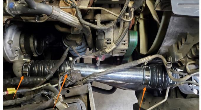
6. Place shop towels or a container under the transmission cooler line connections to catch the fluid that will leak out. Then, remove the dust covers from the transmission cooler line connections and disengage the connections. Properly dispose of any transmission fluid.
