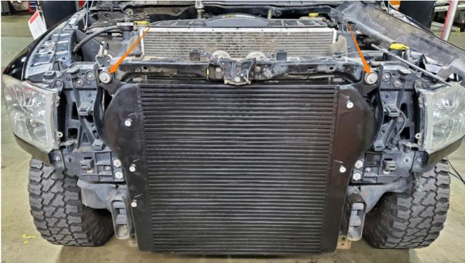
**9.** Remove the clamps that secure the intercooler pipe boots to each side of the intercooler.
