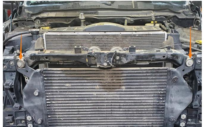
3. Remove the four (4) bolts securing the grille to the vehicle. Then, remove the grille from the vehicle by pulling it away from the vehicle to disengage the clips securing the bottom.
