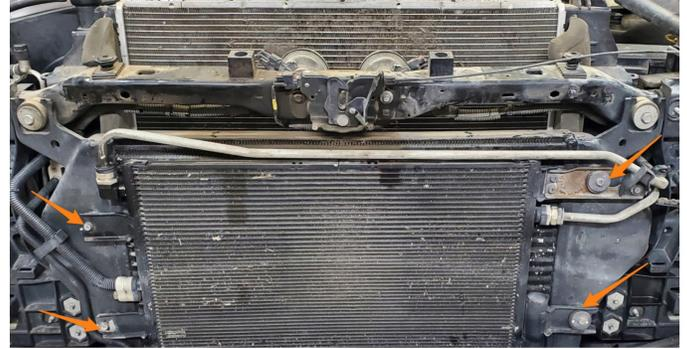
**17.** Reinstall the bumper, plastic shrouds, & grille by reversing the removal steps. Check the transmission fluid level before driving the vehicle and top off if needed. The A/C system can be recharged by most mechanics. The installation is now complete.
