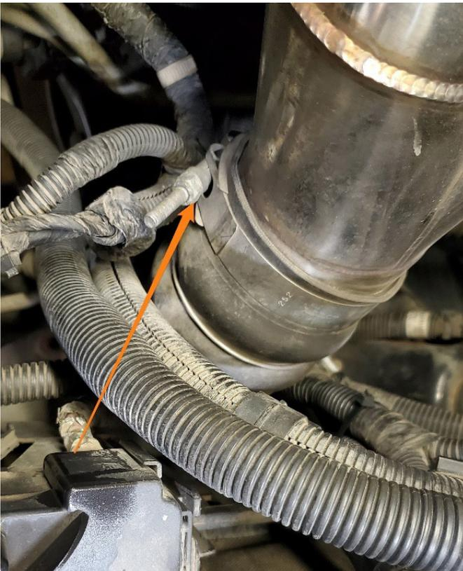
5. **BE SURE THE REFRIGERANT HAS BEEN PROPERLY RECOVERED BEFORE PERFORMING THIS STEP.** Remove the two (2) bolts securing the junction of the A/C condenser lines. Then, remove the one (1) bolt securing the junction to the intercooler.
