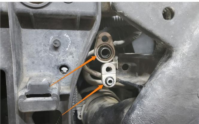
**12.** Remove the clamps securing the stock intercooler pipe boots to the turbo and the intake elbow, and remove the stock pipes and boots from the vehicle.
