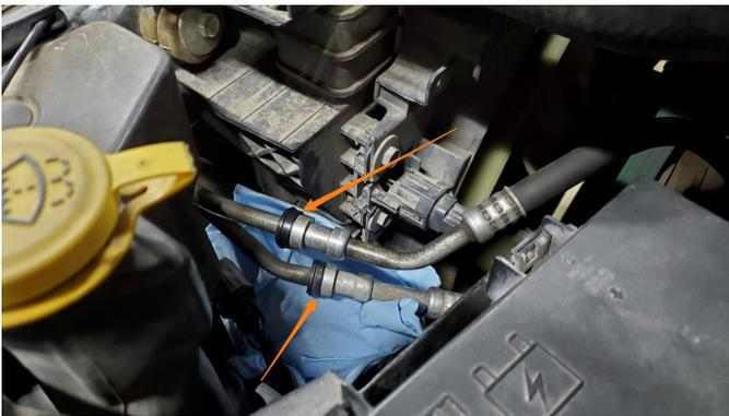
**16.** Reconnect the transmission cooler lines and reinstall the dust caps onto the fittings. Then, replace the seals at the A/C condenser line junction with new seals and reconnect the A/C condenser lines with the two (2) bolts removed in step 5. The bolt that mounted the junction to the stock intercooler will not be reused. (Image on right)
