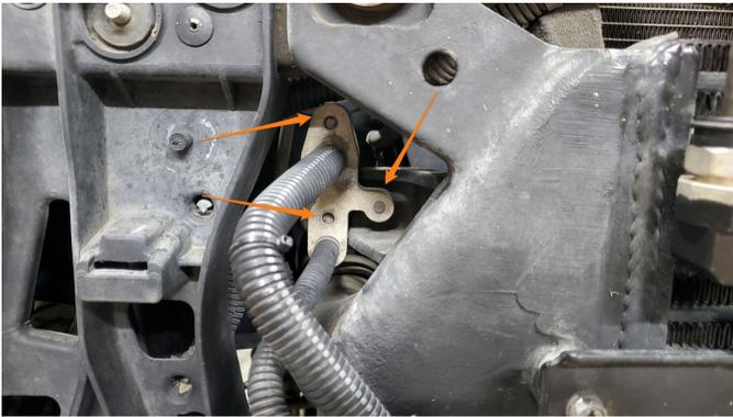
**15.** Reinstall the A/C condenser/transmission cooler and lines and secure them to the intercooler with the four (4) bolts that were removed in step 8.
