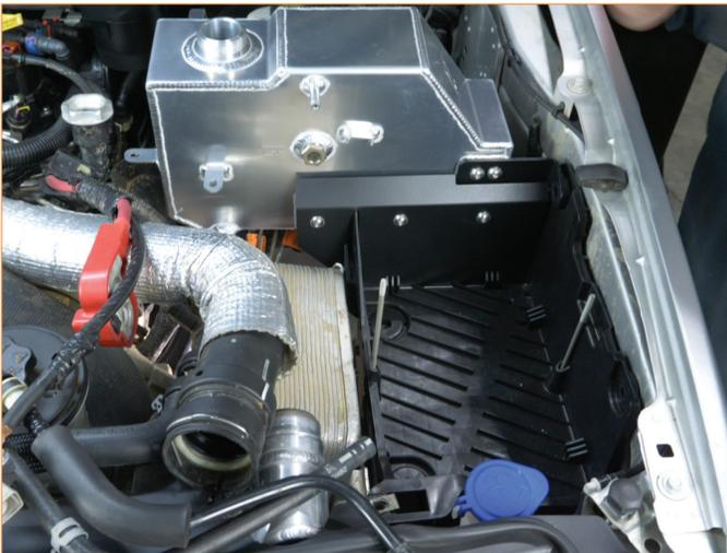
26. Adjust the degas tank so that it is level and then tighten the 5x allen bolts. (5x 5mm allen bolts).
