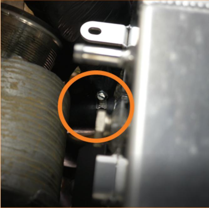
**29.** Install the vacuum hub lock solenoid, vacuum regulator, and vacuum manifold to the rear of the degas tank. (1x 2.5mm allen bolt).
