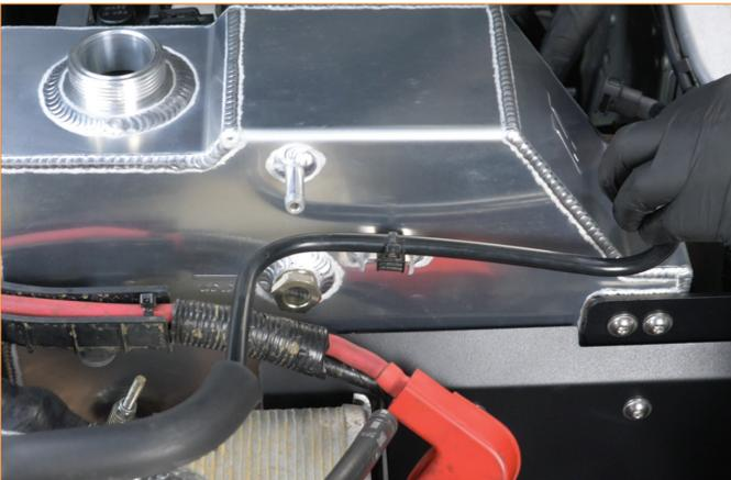
34. Connect the upper hose to the degas tank. (1x spring clamp).
