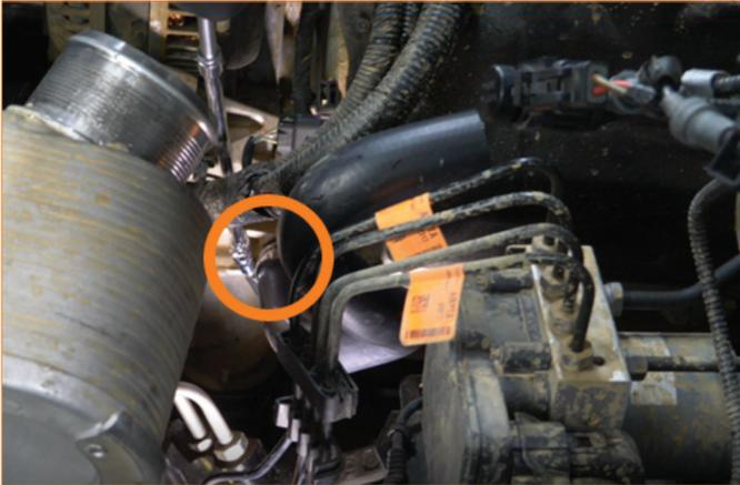
25. Reinstall the battery tray into the vehicle. (4x 13mm bolts).
