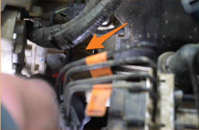
16. Mark the battery tray as shown in the image below. This is where the battery tray must be cut to remove the stock degas tank.
