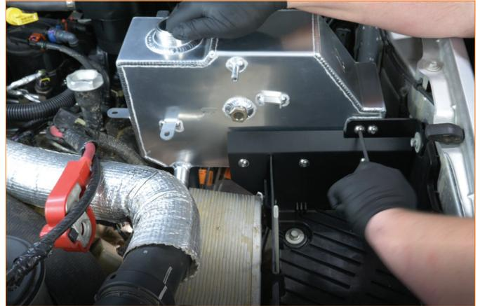
27. Reinstall the intercooler to the side of the battery tray. (2x 13mm bolts).
