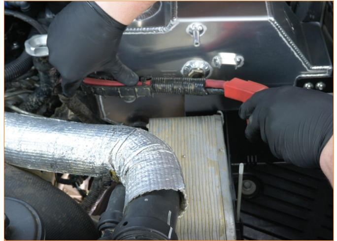
**31.** Reinstall the hot-side intercooler pipe.
