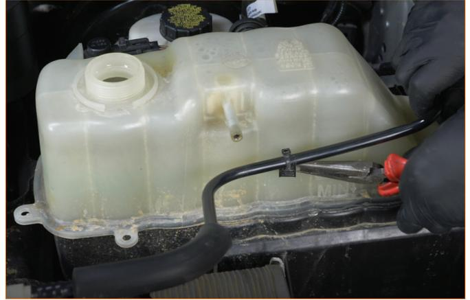
10. Disconnect the vacuum supply hose from the vacuum manifold attached to the rear of the primary degas tank. (1x quick-disconnect fitting).
