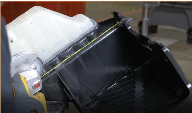
18. Using a reciprocating saw, remove the support ribs from the bottom side of the stock degas tank.
