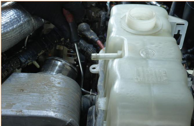
13. Remove the bolts securing the intercooler to the battery tray. Once the bolts are removed, lift the intercooler to unseat it from the battery tray, then push it towards the engine and set it back down. (2x 13mm bolts).
