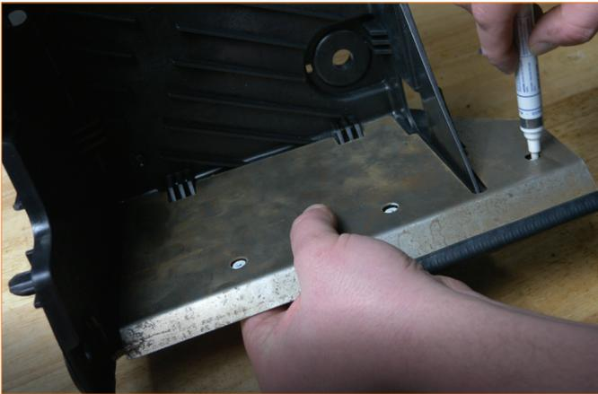
22. Attach the MM2356-02 bracket to the MM2356-01 degas tank using the 2x short 5mm allen bolts. Leave these bolts loose. (2x short 5mm allen bolts).
