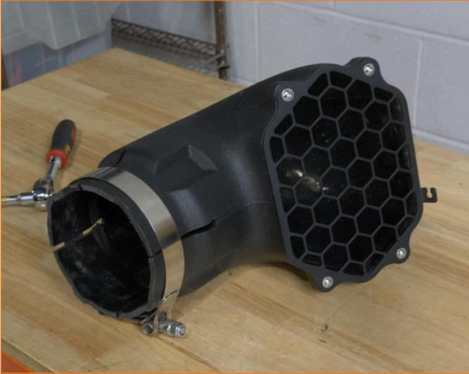
19. Install the snorkel head assembly. Adjust for levelness and orientation, then tighten the t-bolt clamp. Slip the protective rubber cap over the exposed thread on the T-bolt clamp.
