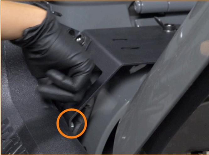
14. Attach the snorkel to the second bracket installed on the fender with 2x M4 button head flanged bolts. **DO NOT FULLY TIGHTEN THESE BOLTS.**
