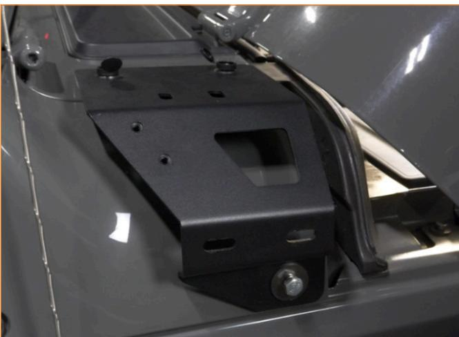
11. Install the smallest bracket onto the large bracket (2x 14mm M6 bolts, 2x M6 flat washers, 2x bolt caps). **DO NOT FULLY TIGHTEN THESE BOLTS.**
