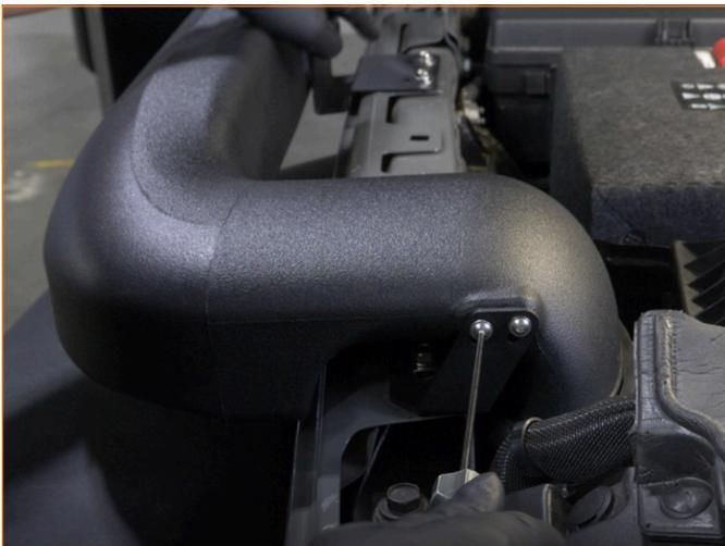
15. Check snorkel clearance with passenger side mirror with door fully open, and clearance with hood cutout when the hood is fully closed and latched, adjust the snorkel assembly accordingly and fully tighten all fasteners.
