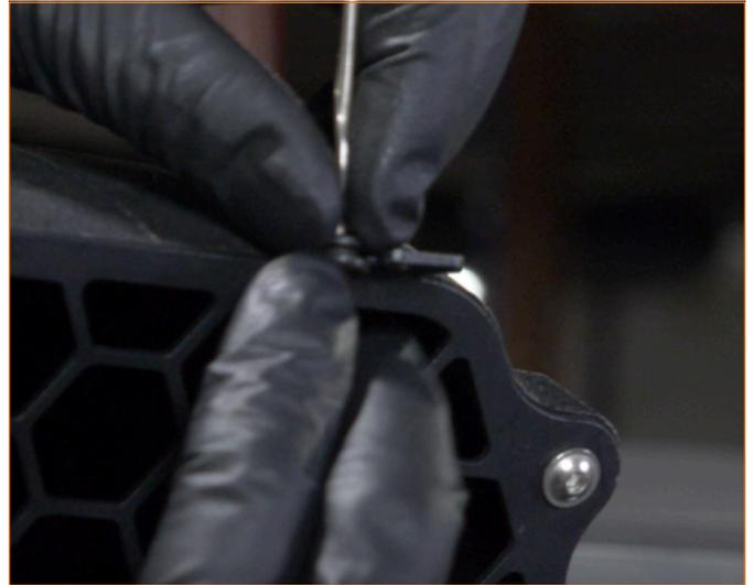
21. Install the rubber hood bezel temporarily. It should be able to move along the cutout on the hood.
