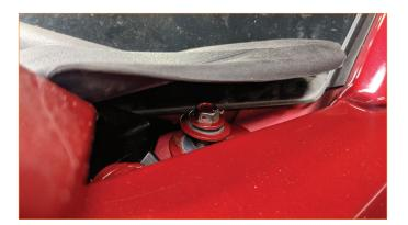
> Remove 3x bolts along the top of the fender.
