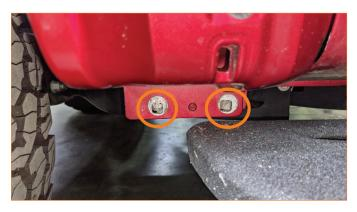
> Pull out the black foam located inside the fender and toward the door to expose the bolt underneath.
