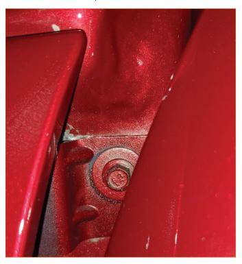
> Lift the corner of the cowl to expose the bolt underneath.
