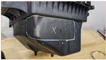
> Reassemble the air intake. Remove the stock fresh air duct and seal the port with provided rubber plug. Note that the plug must be sealed with RTV, silicone caulk or butyl tape if intend to use for water fording. Reinstall the air intake back on the vehicle.
