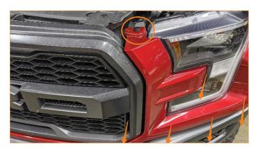
06. Remove the headlight bracket. Remove 6x fasteners from the front and side of the bracket, then release the marker harness from the bracket. Pinch the clip circled just above the bolt to release it and remove the bracket.
