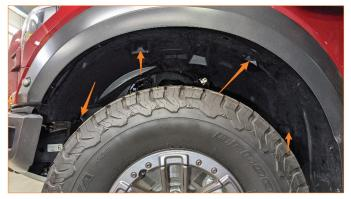
**05.** Remove the headlight trim piece. Remove 1x pop clip then pull the trim piece forward along the edges to release the clips.
