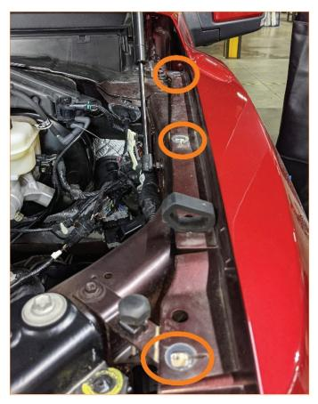
> Remove the one bolt under the headlight.
