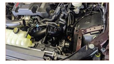
02. Release all harness clips from wheel well liner, push them toward the firewall and secure with provided zip ties. Area indicated by the arrow must be free of wire harnesses. Release the thick main harness wire loom that runs along the fender frame, lift it up and secure with provided tree clip zip tie.
