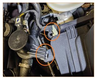
Lift the airbox straight up to disengage the 2x rubber grommets.
