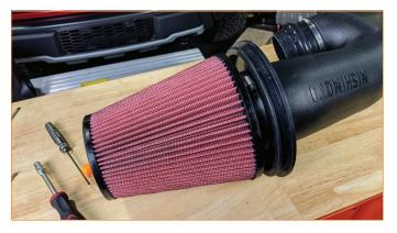
**7.** Transfer the IAT sensor from the stock intake tube to the Mishimoto intake tube. Attach the 2x silicone couplers to the intake tube, secure with 2x worm gear clamps (7mm socket).
