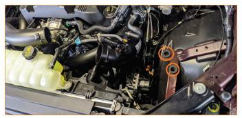
**5.** Install the 2x brackets and 2x pegs onto the Mishimoto intake airbox, as shown in the pictures below. Use the two larger M6 flat washers on the pegs.
