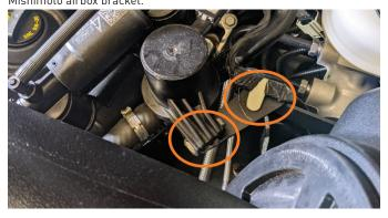
16. Tighten all 4x worm gear clamps on the 2x silicone couplers.
