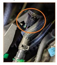
**15.** Secure the vacuum reservoir and harness tree clips to the Mishimoto airbox bracket.
