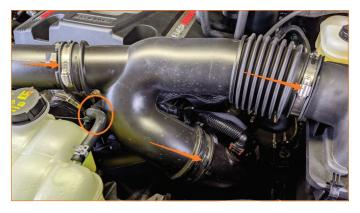
**3.** Unclip the 2x tree clips holding the brake booster vacuum reservoir and electrical harness
