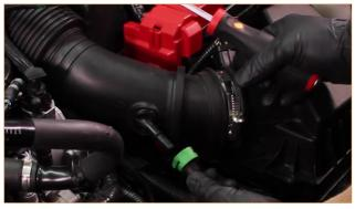
**06.** Loosen the clamps that secure the rubber intake hose to the airbox and the intake tubing. Then remove the rubber intake hose from the vehicle.
