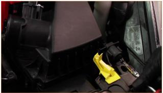
**09.** Separate the air intake duct from the radiator support by prying up on the edge near the center of the duct. Remove the air intake duct and airbox as one unit by pulling the airbox upward. The airbox is secured to the vehicle with two rubber grommets.
