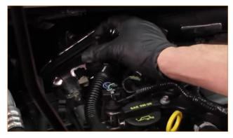
04. Disconnect the crankcase vent hose from the intake tubing by squeezing the knurled tabs where the connector meets the intake tubing. Then swing the vent hose out of the way.
