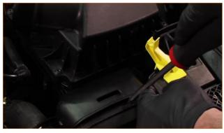
Remove the MAF sensor from the stock airbox. Remove the two Torx screws that secure the sensor, then remove the sensor from the airbox. (2x T20 Torx screws)
