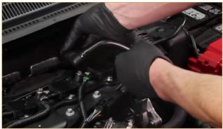
**05.** Disconnect the evap hose from the rubber intake hose. Pry the green locking tab away from the connector to release it, then pull the hose off the port.
