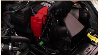
**08.** Remove the airbox isolator bushing. Remove the Torx screw that runs through the center of the bushing. Then remove the bushing by pulling it upward. (1x T20 Torx screw)
