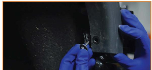
3. Disengage the bumper cap at the sides and along the bottom of the grille. There are a number of tabs just under the grille that will release this piece. Remove the loose bumper cap. (2x 7mm bolts)
