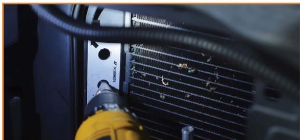
15. Set the line adapters and grommets that are provided in your kit into the recently drilled holes.
