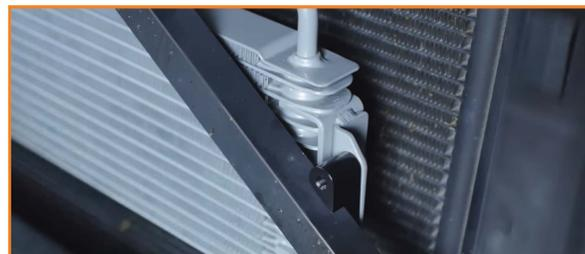
13. Secure the transmission cooler with your mounting hardware. If the cooler is crooked and needs to be adjusted, loosen the button head bolts on the backside of the cooler brackets to adjust its position. (2x brackets, 4x Allen bolts)
