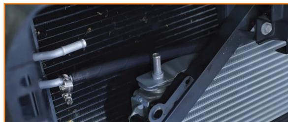
18. Install the short hose to the top port where the holes were drilled and the other to the closer transmission cooler port. (2x worm gear clamp)
