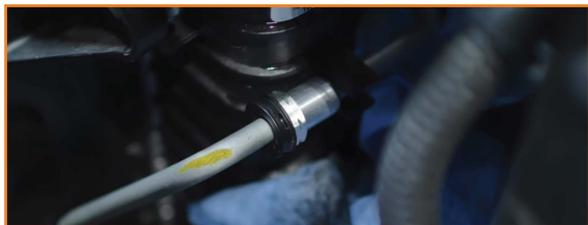
17. Install the long hose to your transmission cooler. One end will go to the bottom port where the holes were drilled and the other to the cooler's furthest port. (2x worm gear clamp)
