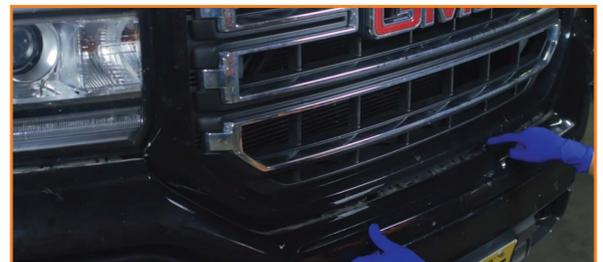
4. Take out the bolts that secure the grille. This includes all hardware along the bottom and top. (8x 10mm bolts)
