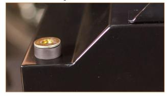
10. Locate the two threaded holes on the inside edge of the radiator support. Install the supplied isolator bushing to the hole that is closer to the center of the vehicle. (1x isolator bushing)
