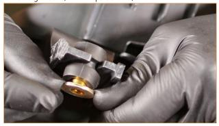
06. Install the MAF sensor to the Mishimoto MAF housing, and secure it with the provided hardware. (2x 2.5mm Allen bolts)
