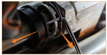
10. Unbolt stock transmission cooler and un-clip lower shield by pulling down on the shield. Remove longer transmission cooler line at the same time as the stock transmission cooler if more clearance is needed (2x 10mm bolts).
