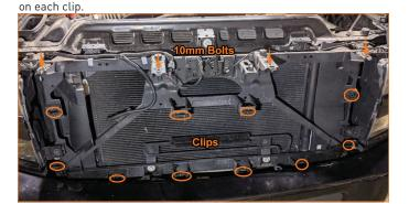
04. There are 10x clips that mount the grille, remove by pulling firmly
