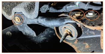
07. Remove bumper bolts, and slide bumper forward to remove (4x 18mm bolts, locations shown without bumper).
