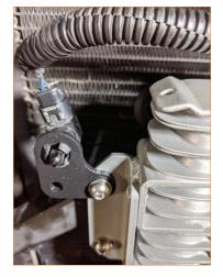
**13.** Install mounting brackets using stock transmission cooler mounting bolt locations and hardware, clip lower shield to brackets with supplied tree clips. Install P-clip around transmission line as shown. Refer to product diagram for bracket assembly (4x 2.5mm hex socket bolts, 1x 2mm hex key w/ 7mm nut for P-Clip).
