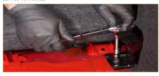
04. Lower the Mishimoto strut brace into place over the seat mounts. Secure the strut brace and the seat mounts using the hardware you just removed. (2x T50 Torx bolts)
