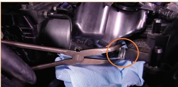
08. Remove the two rubber bushings from the stock expansion tank, and transfer them to the Mishimoto expansion tank.
