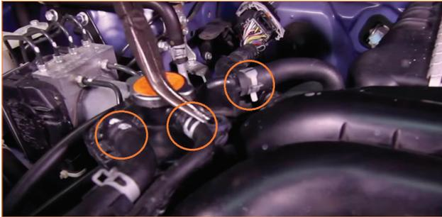
06. Remove the bolt that holds the expansion tank in place. (1x 12mm bolt)
