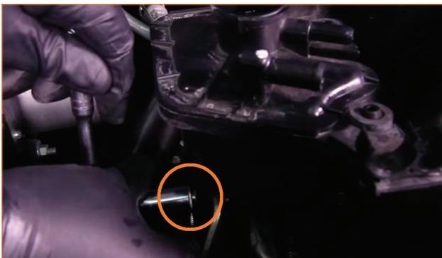
07. Lift the expansion tank to unseat it from the pegs. Locate the lower hose on the expansion tank, compress the spring-clamp that secures it, and slide the clamp down the hose. Then disconnect the hose from the expansion tank.
