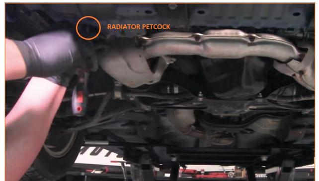
04. Tighten the petcock on the radiator once the coolant has drained below the expansion tank.
