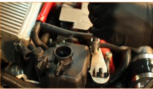
4. Remove the final nut holding the expansion tank in place. [1x 12mm nut]
