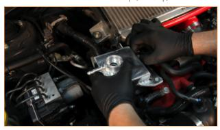
2. Reinstall the bolts on the expansion tank. (2x 12mm bolts)
