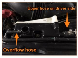
03. Remove the bolts securing the tank to the fan shroud. (2x 10mm bolts)
