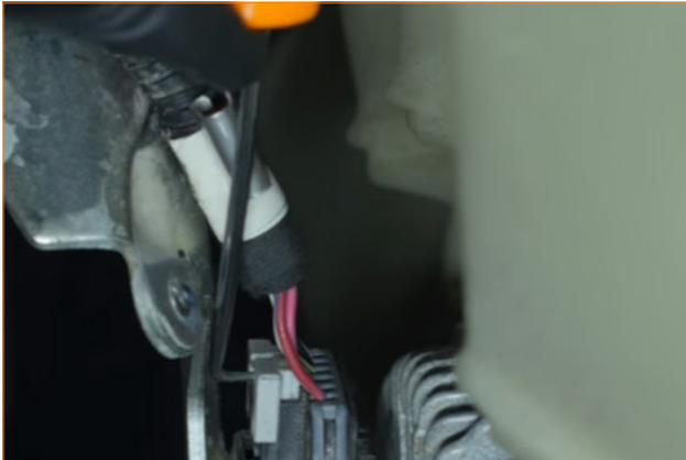
12. Remove the bolt that secures the retainer for the fan clutch harness, and then remove the retainer. (1x 10mm bolt)
