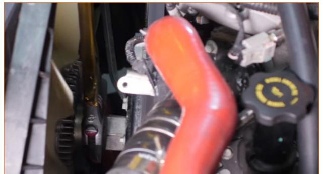
14. Loosen the fan by hand to remove it from the crankshaft drive pulley.
