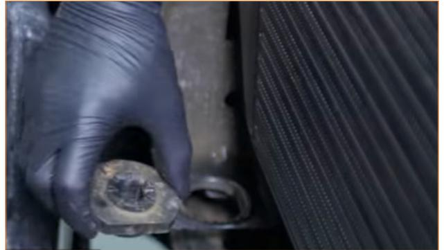
24. Remove the two upper mounting bushings from the factory radiator. Push the collar out of the bushing, and then remove the bushing. Now transfer these bushings to the Mishimoto radiator.
