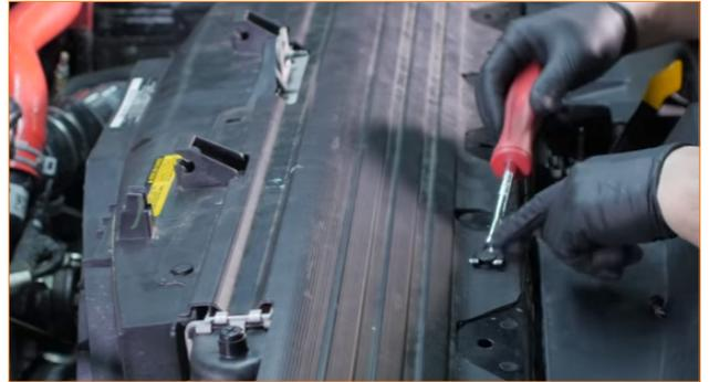
09. Separate the transmission cooler lines from the clips that secure them to the fan shroud.
