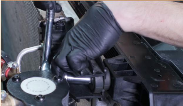
20. Loosen the clamps that secure the cold-side intercooler pipe to the intake and the intercooler. Then remove the cold-side intercooler pipe. (2x 11mm T-bolt clamps)
