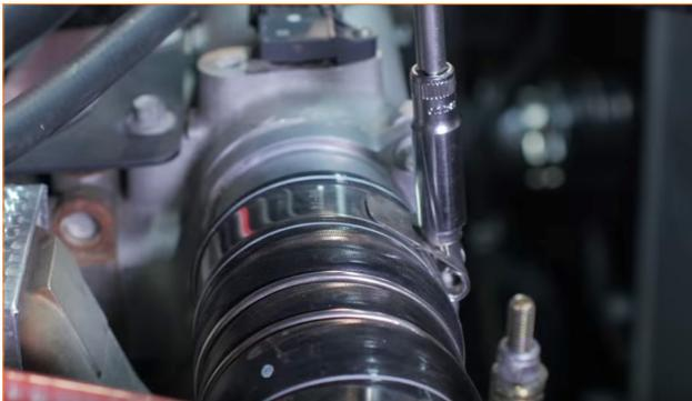
21. Loosen the clamps that secure the hot-side intercooler pipe to the turbo outlet and the intercooler. Then remove the hot-side intercooler pipe. (2x 11mm T-bolt clamps)
