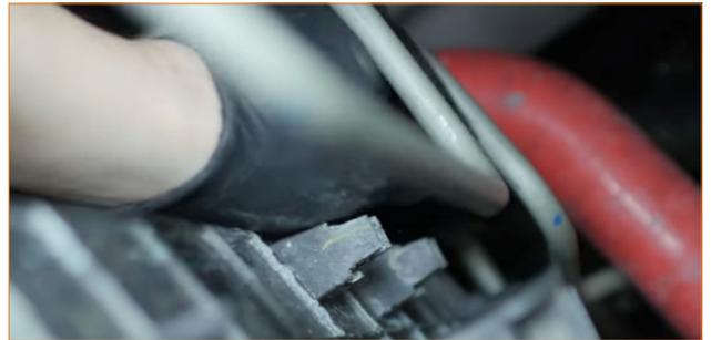
10. Remove the five bolts that secure the fan shroud to the radiator. (5x 8mm bolts)
