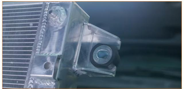
25. Remove the five clip nuts from the stock radiator, and transfer them to the Mishimoto radiator. Use a screwdriver to bend the tang on the clip nut to retain it on the radiator. (5x clip nuts)
