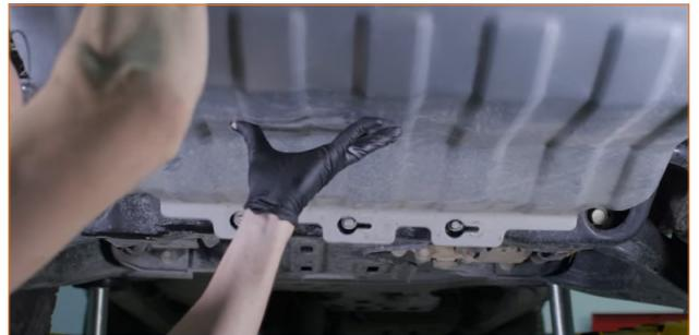
03. Remove the four tree clips that secure the air diversion panel to the underside of the fan shroud. (4x tree clips)
