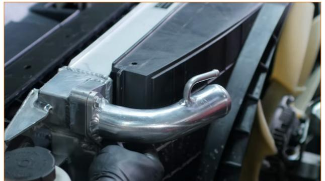
38. Reinstall the hot-side intercooler pipe. Lower the pipe into place and install it over the turbocharger outlet first, and then to the intercooler inlet. Now secure the pipe with the clamps. (2x T-bolt clamps)
