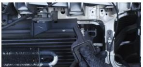
15. Separate the MAF sensor and induction hose from their connections on the intake pipe.
