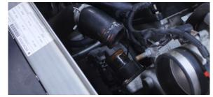
20. Compress the clamp on the upper radiator hose and move it down the hose. Then separate the hose from the radiator. (1x spring clamp)
