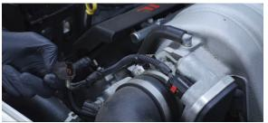
16. Loosen the clamps on each end of the intake pipe where it connects to the throttle body and filter. Our loaner vehicle had an aftermarket intake installed. Expect that yours will look different compared to the one shown here. (2x worm gear clamps)
