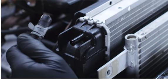
25. Remove the passenger-side radiator shrouding. (2x pop-clips)
