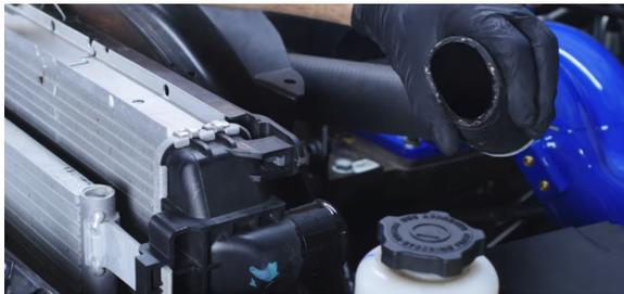
18. Loosen the clamps securing both ends of the hot-side intercooler pipe. Lift the pipe up through the engine bay to remove it.
