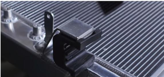
30. Lower the Mishimoto Radiator into the engine bay. Watch for the AC lines and be sure to engage the rubber isolator bushings on the bottom with the crash bar. For older models, connect the
