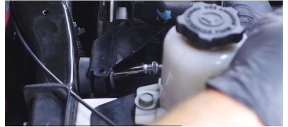
21. Two bolts hold the transmission cooler in place. Remove these bolts, along with the mounting bolt connecting the cooler to the radiator.
