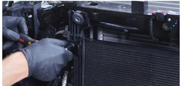
15. Remove the plastic bracket that was formerly securing the AC condenser on the driver side. (2x 13mm bolts, 2x 10mm bolts, 1x pop-clip)
