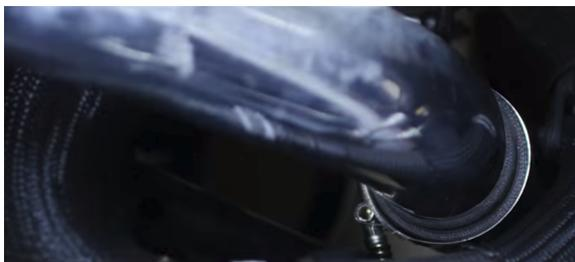
19. Compress the clamp securing the bottom radiator hose to the radiator, and slide the clamp down the hose. Then, separate the hose from the port on the radiator. (1x spring clamp)
