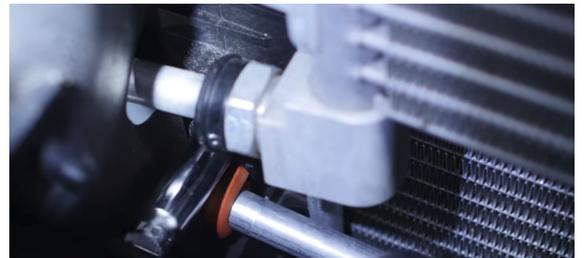
22. Slide the transmission cooler over to get the tabs out from behind the radiator bracket.
