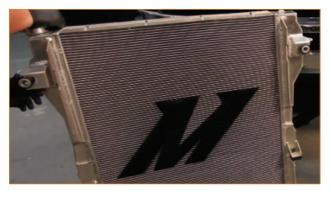
**3.** Carefully put the Mishimoto radiator into place in the engine bay.
