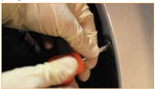
**7.** Remove both side marker housings. After pulling out the housing, locate the clip on the inside of the marker housing slot. Remove this clip on both the driver and passenger sides of the bumper.
